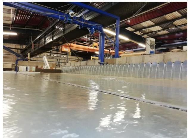
Figure 1. Physical test station of longitudinal inlet grates at the Theodor Rehbock's Hydraulics Laboratory. Left: overview of the model. Right: simulation of a rain event (IWG, 2021).
